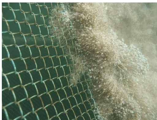
Fig. 1 Four months after deployment in the North Atlantic in June 2009, the plastic structure of this net pen (right) is heavily fouled while the copper alloy mesh remains free of fouling. Source: University of New Hampshire.
