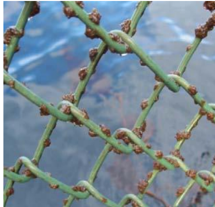
Figure 4: Copper alloy chain link mesh used in aquaculture shown immediately upon retrieval from 15 meter depth after 4 months of immersion. The invertebrates are moving on the surface. Note the complete absence of biofouling and the greenish corrosion protection layer that forms naturally upon exposure to seawater.
